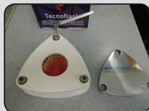
4) Attach top half of flask and tighten all bolts. (Figure 5)
