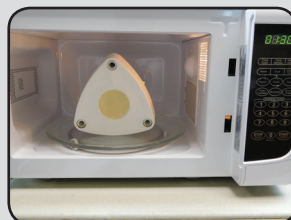
6) After gypsum is set, remove bolts and insert flask in microwave and set timer for 1 minute and 30 seconds. (Figure 7)
